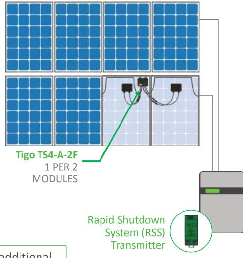
PLC communication with no additional ground wire required
