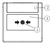
Pressing the black marking (1) breaks the glass pane (3), which triggers the alarm and causes the LED (2) to flash.
