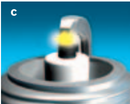
Profiled ground electrode – center electrode
